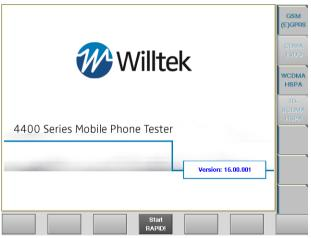
In the Welcome menu, you can immediately start testing GSM mobiles in call mode by pressing the **Calls & Meas.** softkey below the TFT display.
